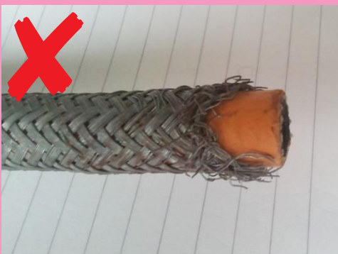
The braided hose is frayed.
